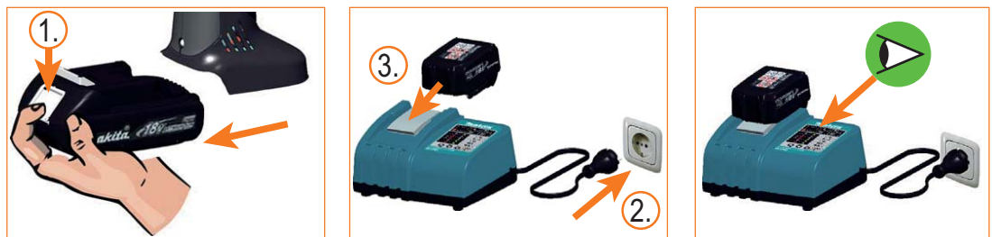
Fig. 5-1 Charging the battery
